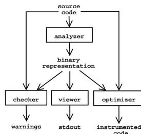
**Fig. 7.** Tool architecture.
