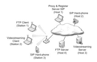
Fig. 3. DTT HotSpot Test-bed; the AP is enhanced with the DTT soft scheduler
