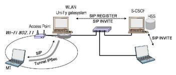
Fig. 9. SIP based WLAN/3G authentication demonstrator layout
