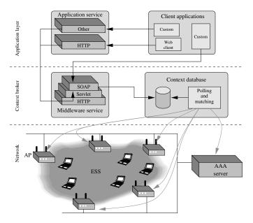
Fig. 10. Block diagram of the context-enhanced service framework
