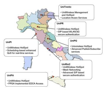
Fig. 1. Overview of UniWireless deployment within the TWELVE project.
