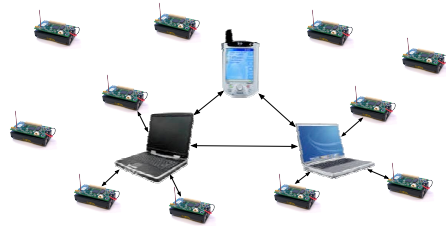
Figure 2. TinyLIME operational scenario: communication occurs between base stations (laptops) and sensors, and between base stations and clients (PDAs). Clients and base stations can also coincide.
